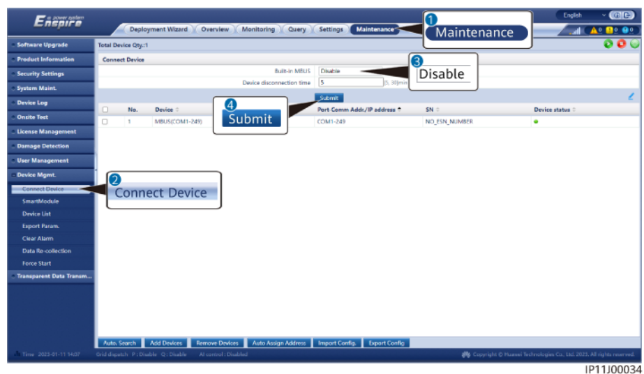
Figure 6-27 Setting parameters for a built-in MBUS module
