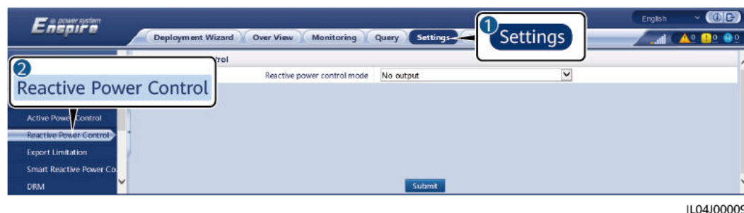
Figure 6-50 Reactive power control
