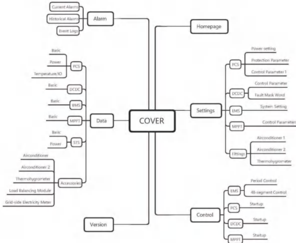
Figure 7-1 HMI Screen menu logical structure distribution diagram
