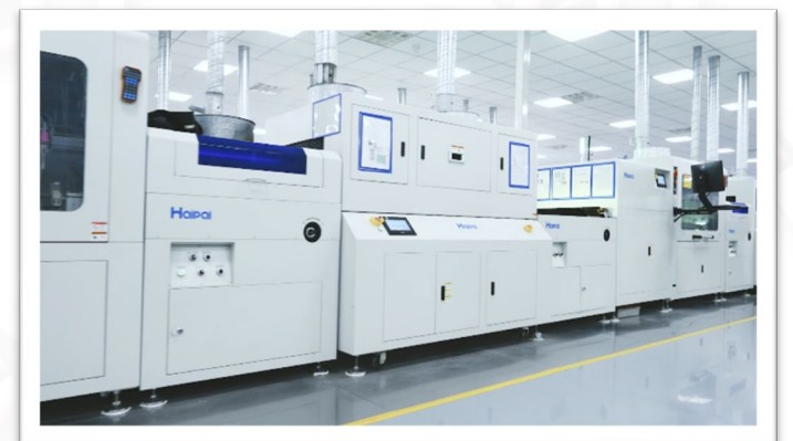
Three-proof Paint Spraying Workshop
