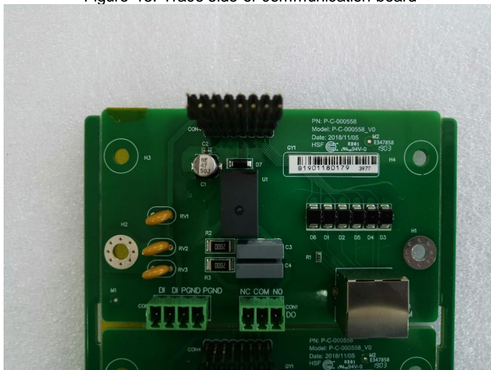
Figure 16. Component side of DIDO Interface board
