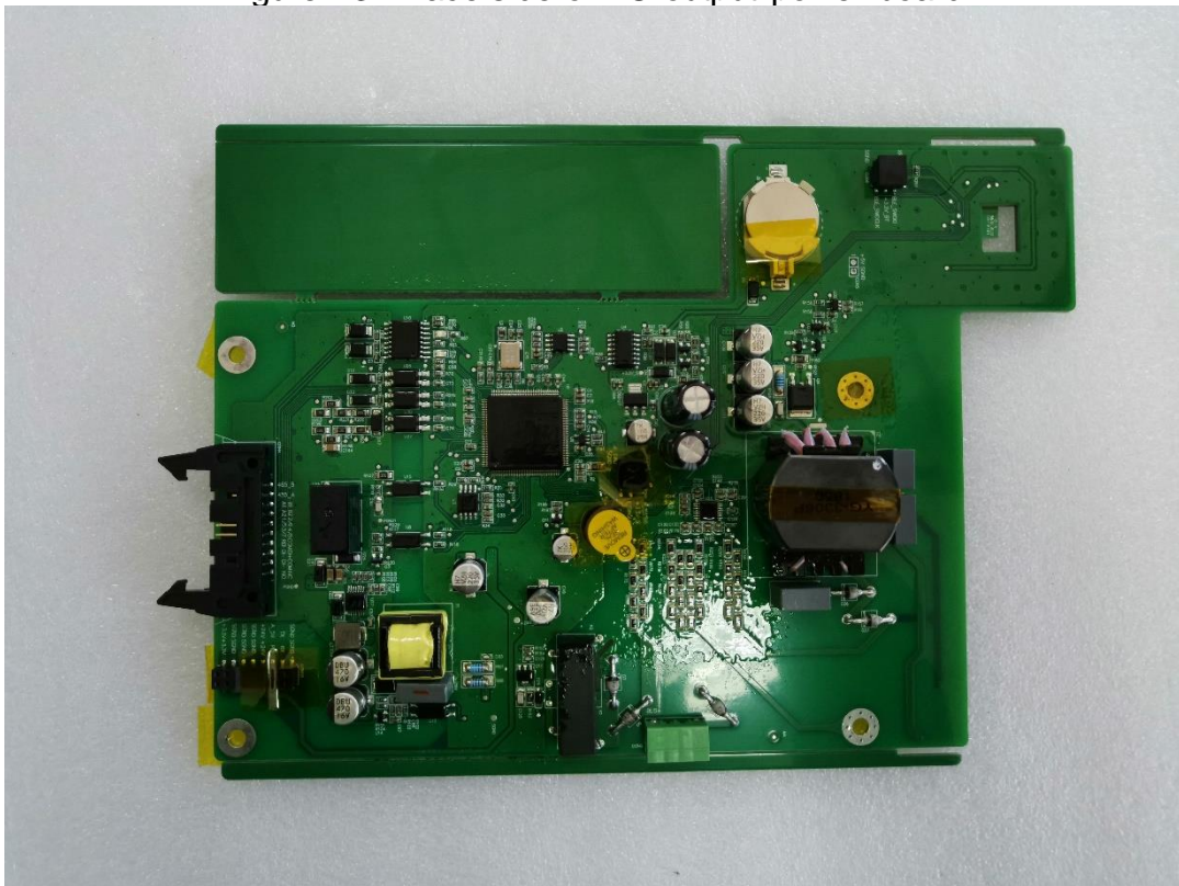
Figure 14. Component side of communication board
