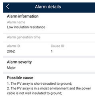
Figure E-1 Alarm details
