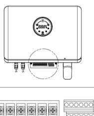
R/L S T/N PE U V W CONTROL OF SORT
