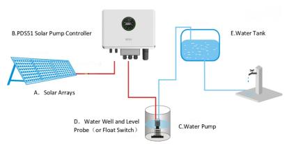
Figure 1-1-1 Solar Pump System
