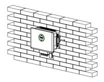
Figure 3-4-3-4 Screw fixing on the side of the controller
