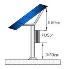
Figure 3-3-2 Installation Location
