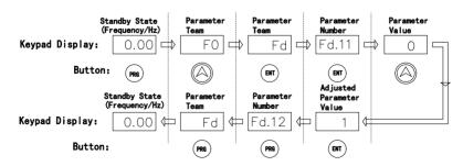
Figure 4-4-1 Schematic diagram of function parameter adjusting
