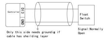
Figure 3-5-5 Wirings of Float Switch
