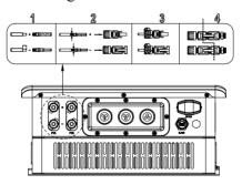
Figure 3-4-5 Connecting component terminals
