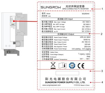
Figure 3-1 Nameplate of Inverters
