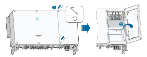
Step 3 Keep the wiring compartment opened during wiring through the limit lever attached to the cover.
