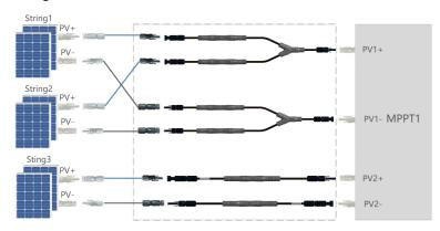
Sungrow can provide Bizlink's Y-branch connector. If necessary, please contact Sungrow to purchase. Customers can also purchase Y-branch connector of the same specification by themselves. The wiring instructions for Y-branch connector are as follows.
