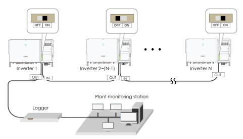
**Figure 5-5** Configuration of dip switch (N $\ge$ 15)
