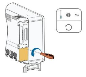
Step 3 Press the hump of the latch hook, unplug the cable connection joint outwards, and loosen the screw on the fan holder.
