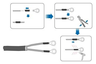
Step 6 Stack the OT terminals on the OT/DT terminal of the AC cables, and fix the cables to corresponding terminals.
