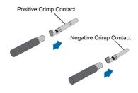
Step 3 Insert the crimped cables into the corresponding connectors until they snap into place. Gently pull the cable backward to ensure firm connection.
