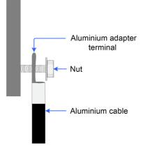
Figure 5-3 Aluminium cable terminal connection sequence
