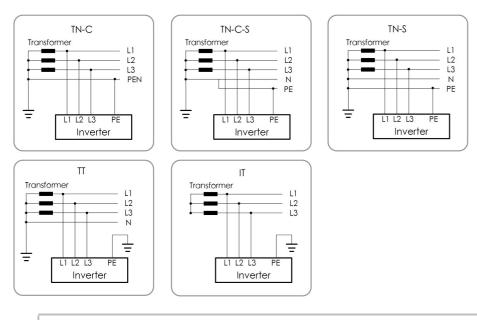
Make sure the inverter is applied to an IT system before enabling the Anti-PID function.
