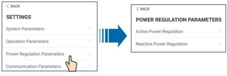
Figure 7-18 Power Regulation Parameters
