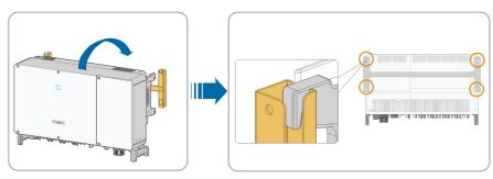
Step 8 Fix the inverter with screws.
