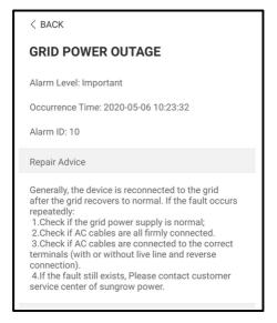
Figure 7-9 Detailed fault alarm info
