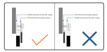
Step 7 Gently pull the cable backwards to ensure firm connection, and fasten the swivel nut clockwise.
