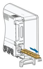
Step 5 Follow the steps above to remove the fan on the other side of the inverter.
