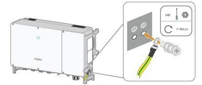
Step 3 Apply paint to the grounding terminal to ensure corrosion resistance.
