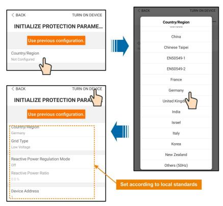
Figure 7-4 Initialization protection parameter
