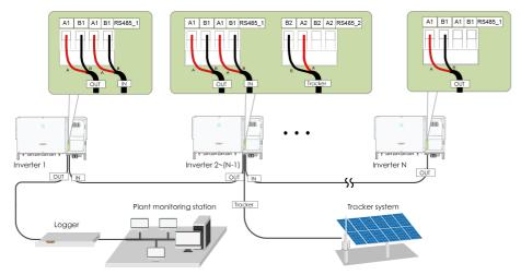
When more than 15 inverters are connected on the same daisy chain, configure the RS485- dip switches of the inverters on two ends of the chain (RS485\_1 is corresponding to SW2, and RS485\_2 is corresponding to SW1), to ensure communication quality.
