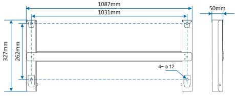
Figure 4-1 Dimensions of mounting-bracket
