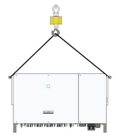
Step 4 Remove the lifting rings and reassemble the sealing screws released in Step 1.
