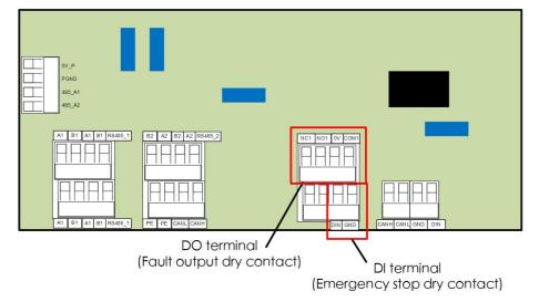
**DO terminal (fault output dry contact):** the relay can be set to fault alarm output, and user can configure it to be a normal open contact (COM&NO) or a normal close contact (COM&NC).
