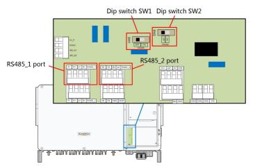
The inverter is equipped with two groups of RS485 communication interfaces for external communication connection.
