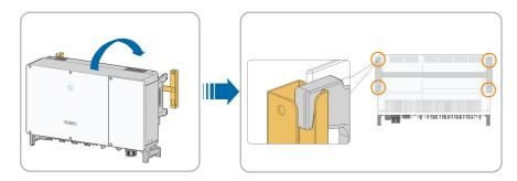
Step 7 Fix the inverter with two M6 × 65 screws.
