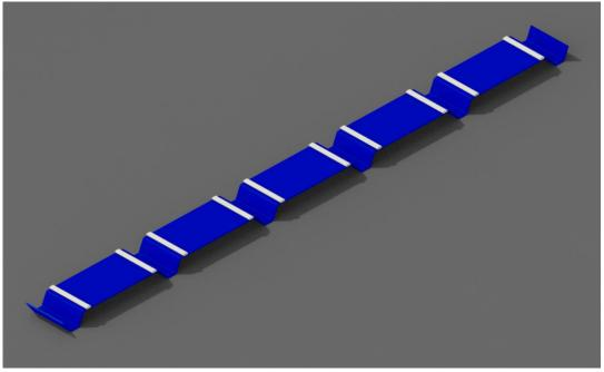
Paste the CS supports along the gluing area and softly press them, keeping the thickness of the glue not less than 3mm.
