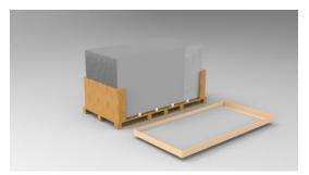
9. Place the box cover open side up and transport the module flat inside the cover to the project designated installation site Place a maximum of two modules in the cover, separated from each other with foam inside the box
