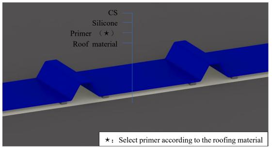
Overlap the crests of 2 adjacent CS supports, and use structural adhesive to paste the lap joint together (as shown in the figure)
