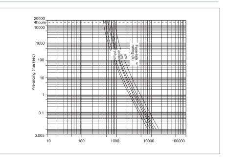
A range of 10x85mm PV fuses specifically designed for protecting and isolating photovoltaic strings. These fuse links are capable of interrupting low overcurrents associated with faulted PV systems (reverse current, multi-array fault). Available in four mounting styles for application flexibility.
